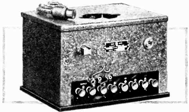
An eliminator for A.C. mains in which provision is made for H.T., L.F. and grid bias. The latter is obtained from a potential divider.
