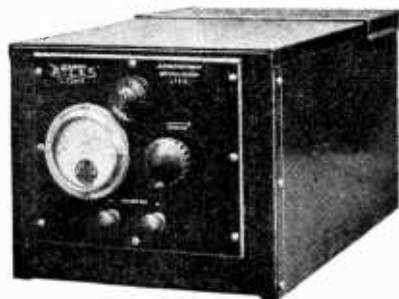
Filament current from A.C. mains: the new Atlas L.T. unit.
