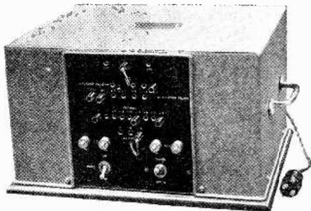
Gambrell complete battery eliminator giving H.T., L.T. and grid biasing potentials.
