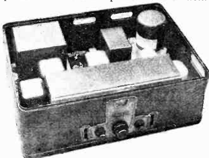
The Crosley Gembox. It is a 5-valve all-mains operated receiver with two neutralised stages and single knob tuning. (Rothermel).
