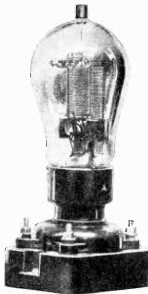
The B.T.H. screened grid valve with 2-volt filament.
